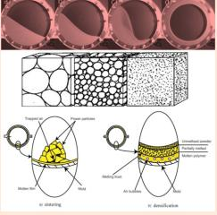
A study shows that there is direc correlation between the number of bubbles in a rotomolded article and its impact performance, with a resulting in lower impact performance. It's no denying that t internal bubbles is a characteristic feature of products manufactured by rotational moulding normally looked after to know whether the part is rotomoulded or not.
