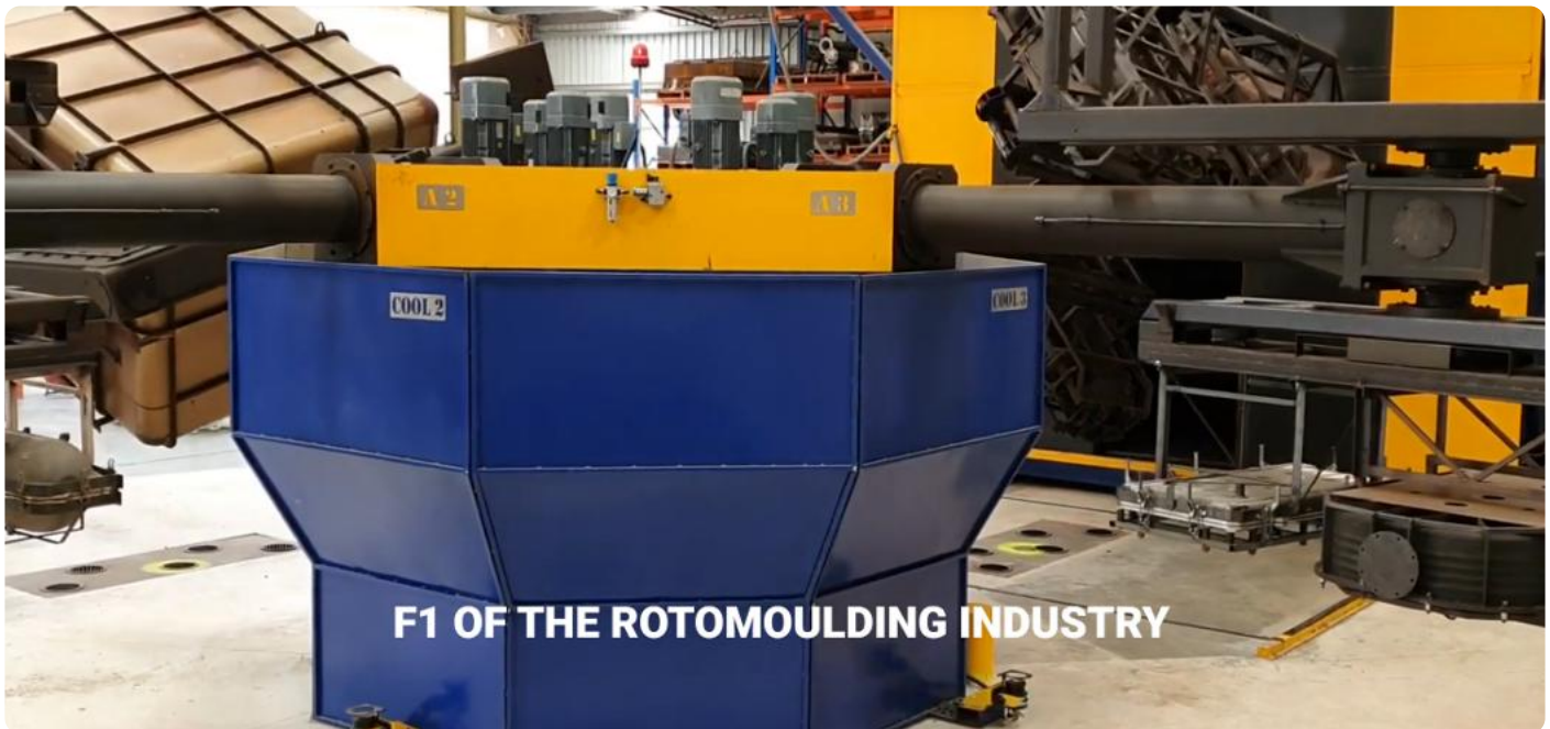
Reinhardt Teknik Rotomoulding Machine in operation
