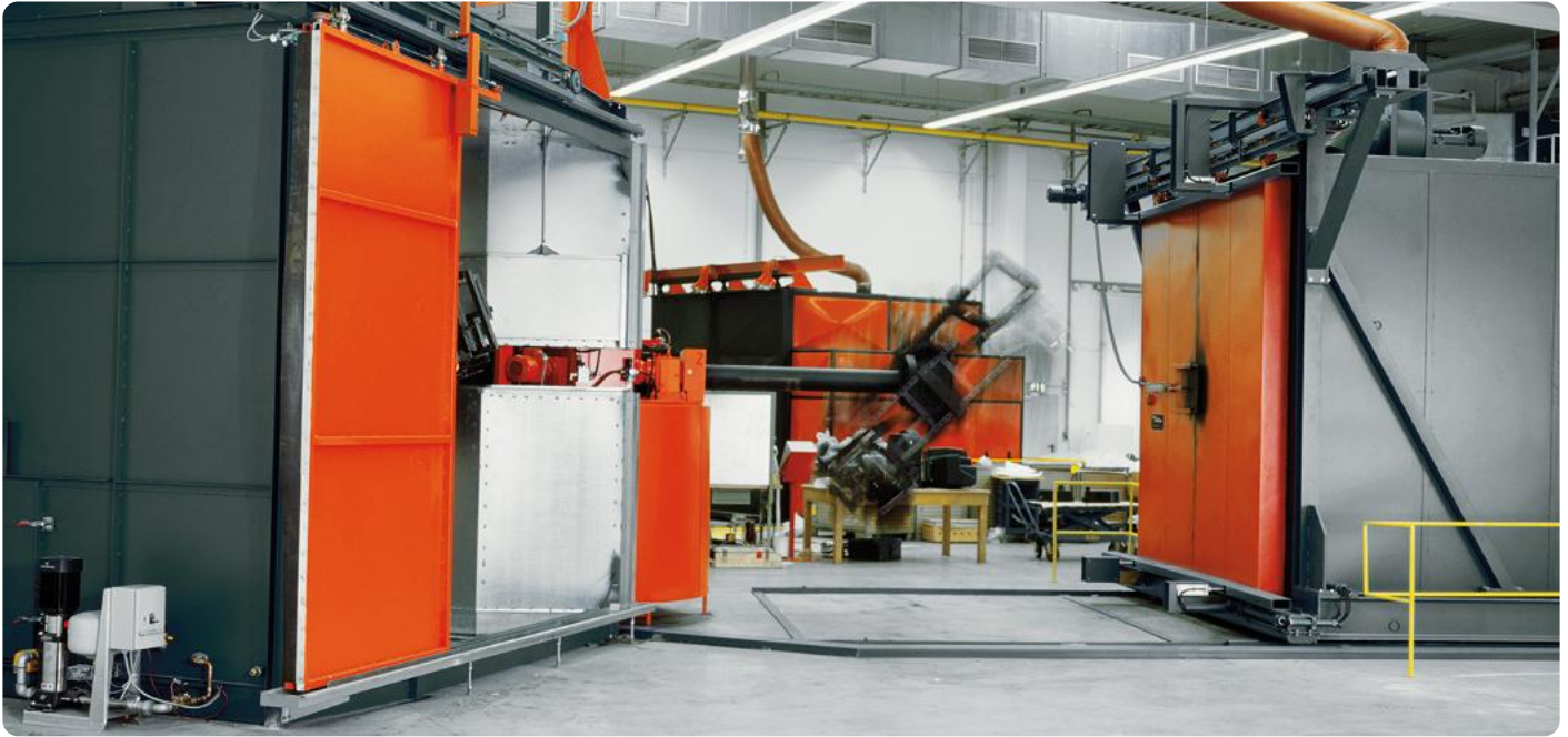
Reinhardt Teknik Rotomoulding Machine in operation
